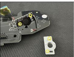
• Place membranes on their respective motherboard connectors. Holes are positioned on the connector to guide your positioning.
