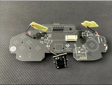
• Remove carefully tapes that keep L, R, Z buttons contacts in place. Wires seems fragile act with precautions
