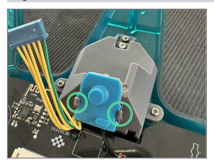
Attach the Z button connector and its membrane onto the stick clips.
