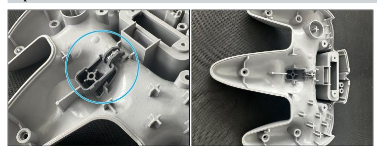
Place the Z button on the bottom shell.
