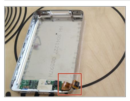
Reconnect the bottom case connector. Before reassembling the iPod.
