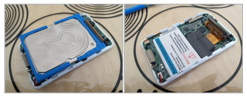
Remove the hard drive with your hand, by holding both the iPod and hard drive connector (hold tight in order to not broke the connector).
